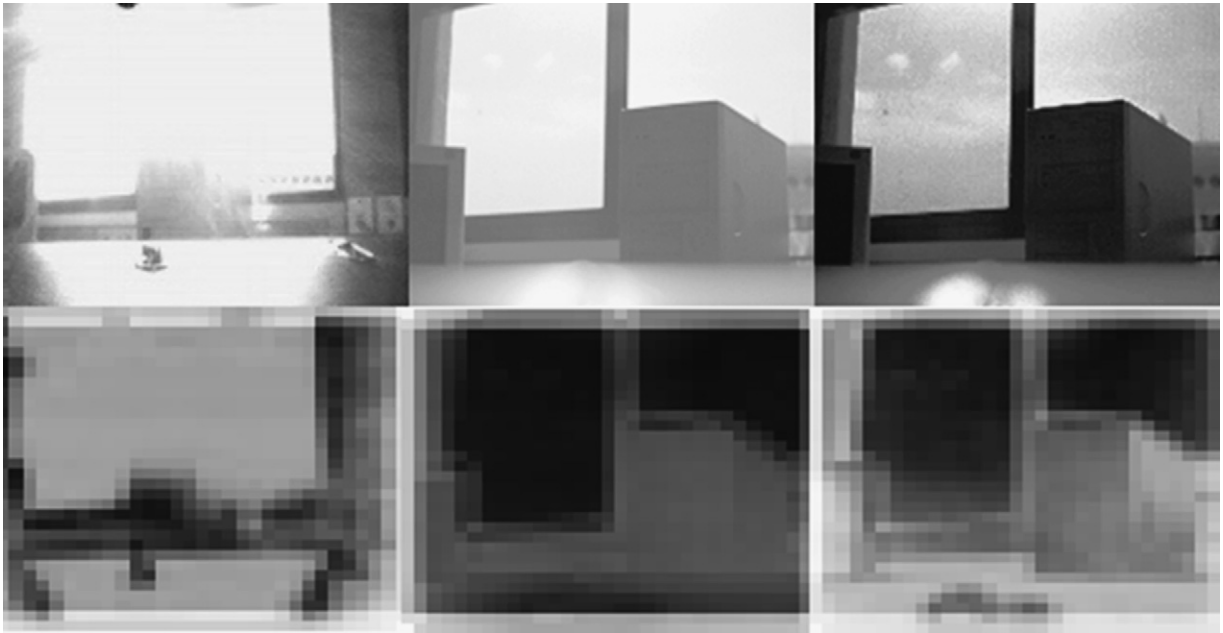
Fig. 3. A view of a window in a shiny day captured by a CMOS camera (upper-left), a logarithmic camera (upper-middle), and equalized view of the logarithmic image (upper-right). The three lower pictures show the result of applying a retina-like processing to its corresponding upper captures.
